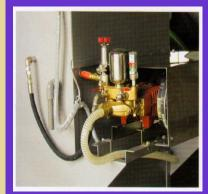
Cleaning Pump of Wedge Screen (Type V ) Middle Pressure 1.2kg/cm²
